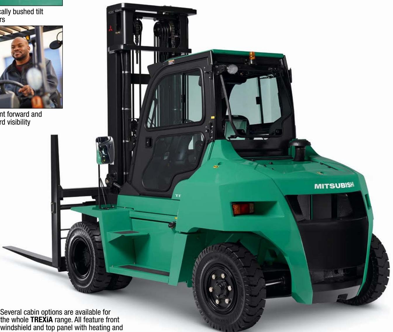
Several cabin options are available for the whole TREXIA range. All feature front windshield and top panel with heating and defogging. A steel door option shown here.
