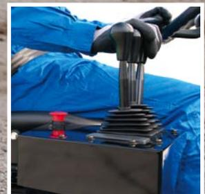
Mechanically isolated ergonomic levers reduce vibration
