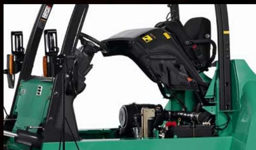
Routine checks and fluid top-ups are made quick and easy with **TREXiA's** RapidAccess design. The seat assembly tilts back effortlessly so the engine compartment is within easy reach. Meanwhile, intelligent engine management heads off trouble by recognising abuse. Further still, scheduled maintenance intervals and oil changes are more infrequent than ever.
