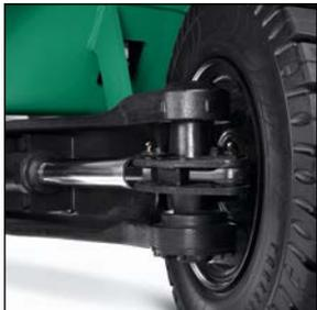
Hydrostatic steering eliminates kickback
