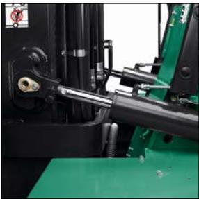
Spherically bushed tilt cylinders
