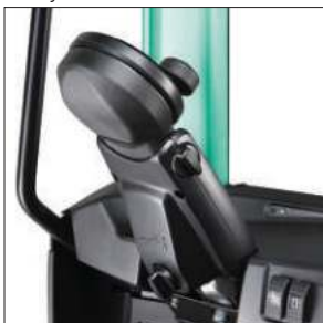
Folding steering wheel console
