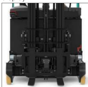
1070 mm width between support legs
