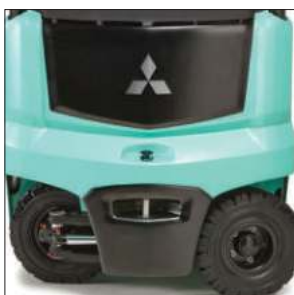
Rear axle steers more than 100 degrees
