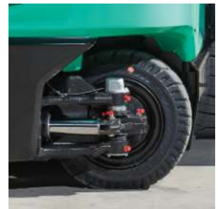
100-degree steering axle
